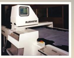
The **BlueSorter** is a visual grading and analysis system for the measurement of wet-blue leather hides/sides and skins. The basic machine comprises of automatic area measurement and substance measurement (optional), with visual quality grading (manual output).
