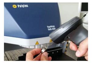
Integrated bar code scanner simplifies sample handling and recipe loading.
