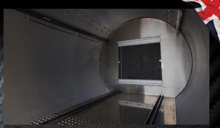
The curing process for composite materials carried out in Roaches autoclaves is fully controlled by the PC based Adaptive Control System (ACS) that has been developed over many years. Using ACS software all the parameters involved in the cycle such as temperature, pressure and vacuum can be programmed and controlled to the most precise level and accurately repeated week after week.
