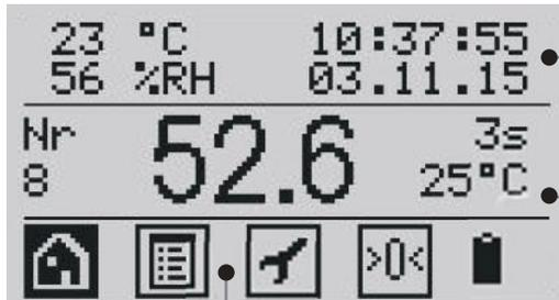
The top section of the display indicates the ambient temperature and humidity, current date and time.
