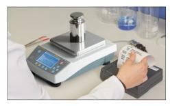
**GLP/ISO record keeping** of weighing data, balance adjustment, etc. with date, time and identification no. etc. Ideal for monitoring and documenting your processes in accordance with your quality management system
